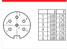
Contact arrangement (Plug-in side)
